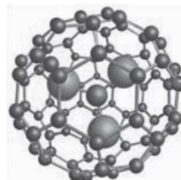
Fig. 2. Metal atoms entrapped within the ‘cage’ of the fullerene
